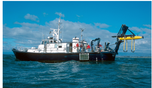
Fig. 1. The MBARI Dorado AUV being deployed from its support vessel the R/V Zephyr .
